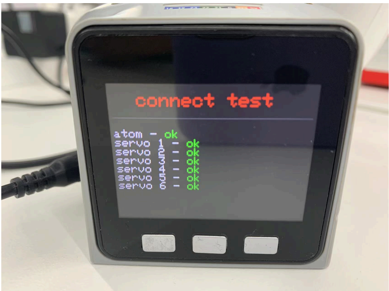
As shown in the figure, the motor connection is in good condition Step 4: Press the B key to start detecting the
