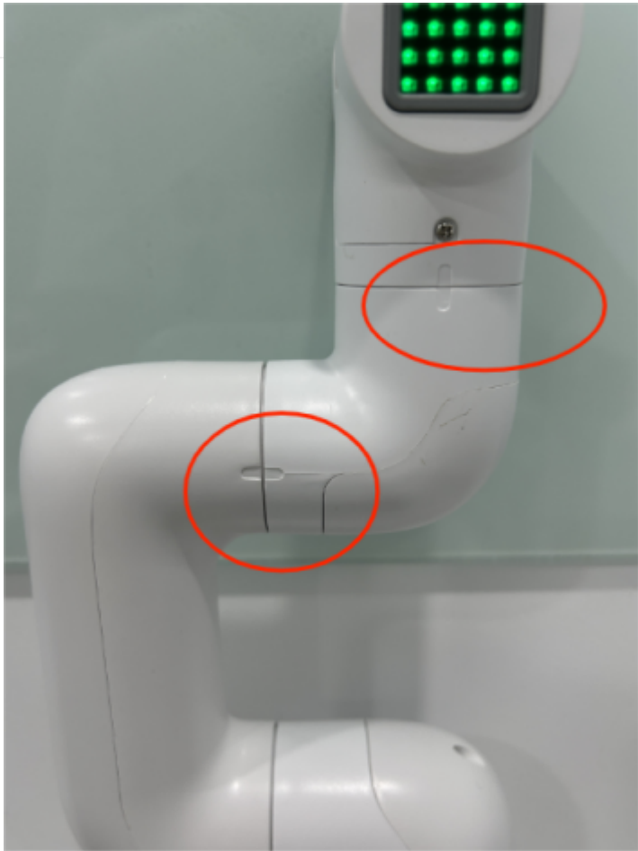
Example diagram of robot arm joint zero position
