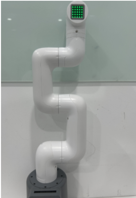
Example diagram of robot arm joint zero position
