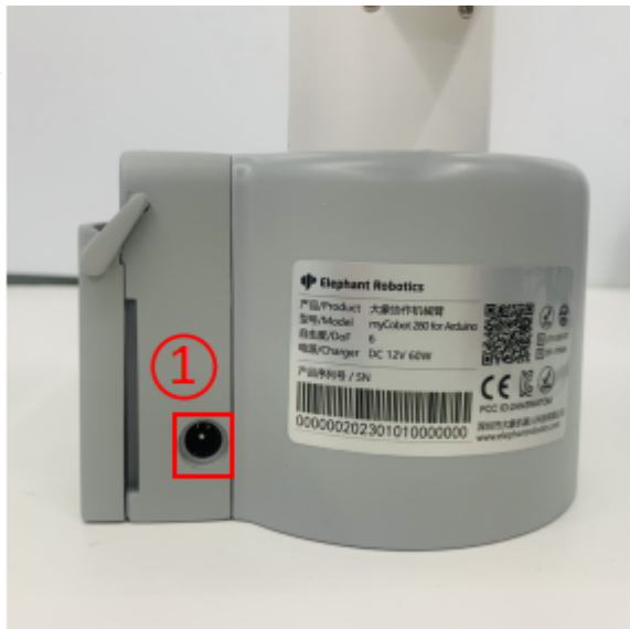
Figure 2.1.8.2-3 Interface on the right side of the base
