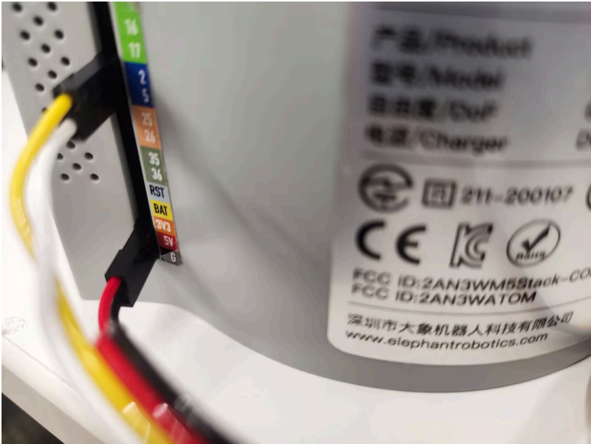
The left side is the suction pump pin, and the right side is the robot arm pin GND -> GND 5V -> 5V G2 -> 23 G5 -> 33
