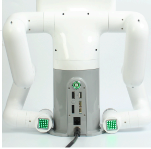
Figure 3-1 Location of the power connector
