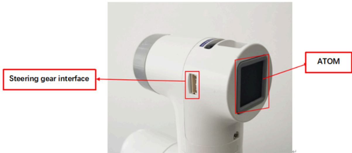
Figure 2-1 Side view of the end of the manipulator
